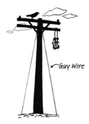
A guy wire and its tower form a right triangle. It is important that all guy wires form congruent triangles so that the tension on each wire is the same.
